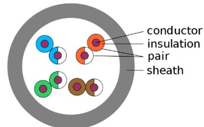
For urban outdoor telephone cables containing hundreds or thousands of pairs, the cable is divided into small but identical bundles. Each bundle consists of
