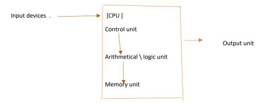
INPUT DEVICES: Computer system use many devices for input purpose. Input devices include the mouse, input pen, touch screen and microphone. Regardless of the type of the devices us all are components for interpretation and communication between people and computer system.
