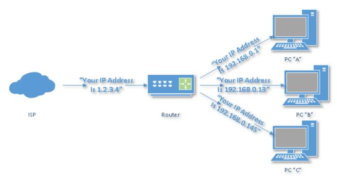
IP address assignments to and through a router.
