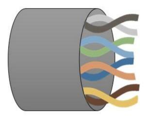
The two wires are twisted in the twisted pair cable which significantly reduces the noise generated by the external source. The **NOISE** here we are talking about is generated when two wires are parallel which causes an increase in
