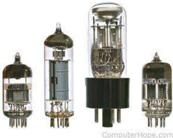
The first generation of computers used [vacuum tubes](#) as a major piece of technology. Vacuum tubes were widely used in computers
