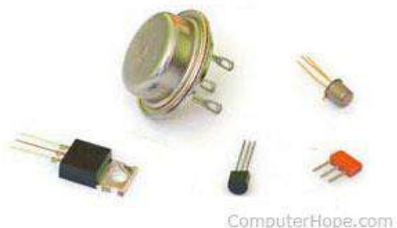
The second generation of computers saw the use of [transistors](#) instead of vacuum tubes. Transistors were widely used in computers from [1956](#) to [1963](#). Transistors were smaller than vacuum tubes and allowed computers to be smaller in size, faster in speed, and cheaper to build.
