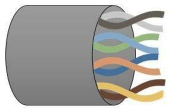
**Shielded twisted-pair (STP) cable** has an additional braided mesh coating or metal foil that wraps each set of insulated conductors. The metal casing intercepts the penetration
