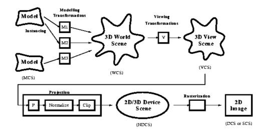
Each stage refines the scene, converting primitives in modelling space to primitives in device space, where they are converted to pixels (rasterized).
