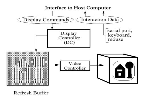
Raster display stores bitmap/pixmap in refresh buffer, also known as bitmap, frame buffer; be in separate hardware (VRAM) or in CPU's main memory (DRAM) Video controller draws all scan-lines at Consistent >60 Hz; separates update rate of the frame buffer and refreshrate of the CRT
