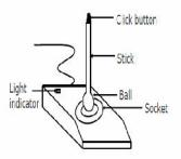
Common y used for video games, flight simulators, training simulators, and for controlling industrial robots
