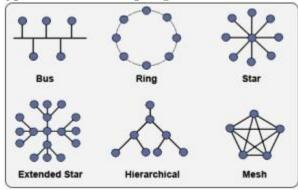
A <u>topology for the network</u> is known to be a layout for the connected devices. This is important because this is used to provide a proper flow of data within the said network. Here are the various topologies:
