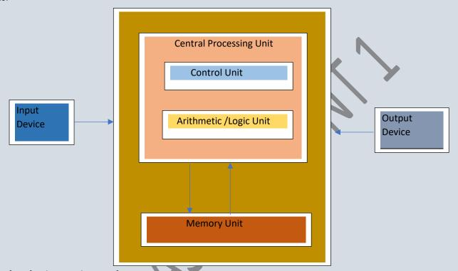
The four fundamental parts of computer are:
