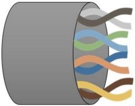
The two wires are twisted in the twisted pair cable which significantly reduces the noise generated by the external source. The **noise** here we are talking about is generated when two wires are parallel which causes an increase in voltage level in the wire closest to the source and also uneven load and damaged signal.
