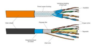
electric or magnetic fields. The idea is that the currents induced in each of the two wires are very nearly equal. The twisting ensures that the two wires are on average the same distance from the interfering source and are affected equally. The noise thus produces a common-mode signal which can be cancelled at the receiver by detecting the difference signal only, the latter being the wanted signal.
