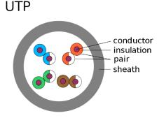
Unshielded twisted pair (UTP) cables are found in many Ethernet networks and telephone systems. For indoor telephone applications, UTP is often grouped into sets of 25 pairs according to a standard 25-pair colour code
