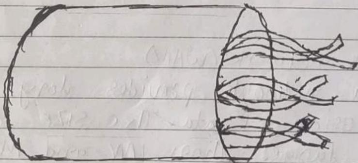
Shielded twisted-pair (STP) cable has an additional braided mesh coating or metal foil that wraps each set of insulated conductors. The metal casing intercepts the penetration of electromagnetic noise. It also can eradicate a phenomenon called crosstalk which is the unwanted effect of one
