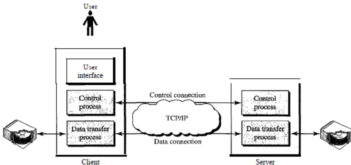
The control connection remains connected during the entire interactive FTP session. The data connection is opened and then closed for each file transferred. It opens each time commands that
