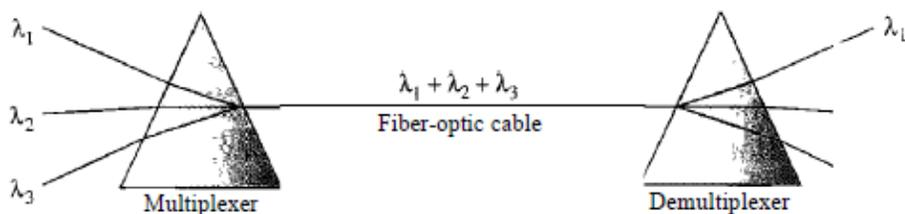
One application of WDM is the SONET network in which multiple optical fiber lines are multiplexed and demultiplexed.
