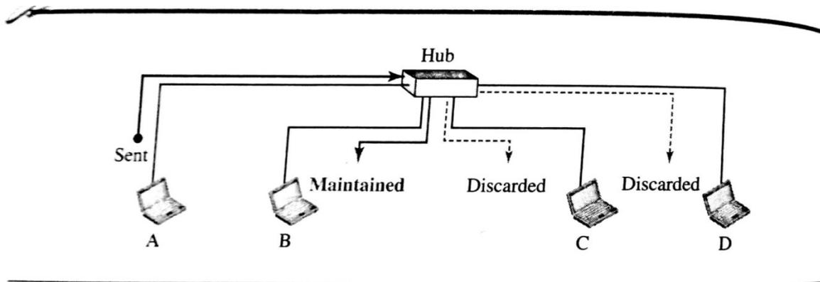
A hub is a physical layer device. They do not have a link layer address and they do not check the link layer address of the received frame. They just regenerate the corrupted bits and send them out from every port.
