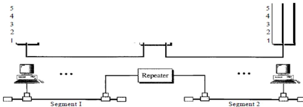
A repeater does not actually connect two LANs; it connects two segments of the same LAN. The segments connected are still part of one single LAN. A repeater is not a device that can connect two LANs of different protocols.
