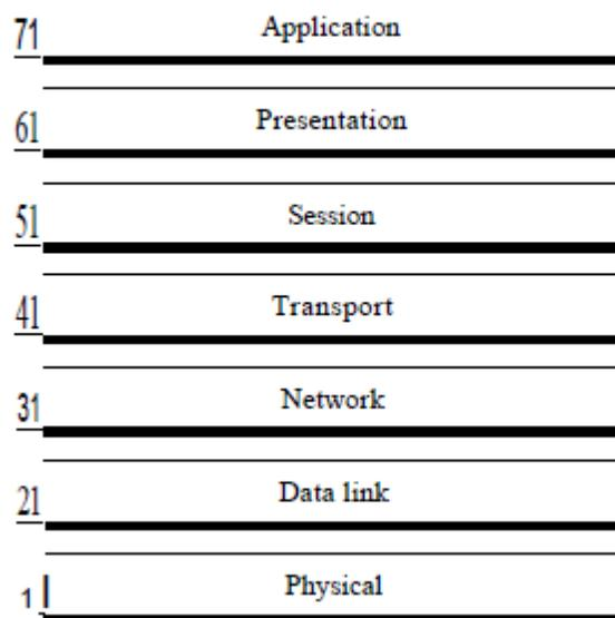
The OSI model is composed of seven ordered layers: physical (layer 1), data link (layer 2), network (layer 3), transport (layer 4), session (layer 5), presentation (layer 6), and application (layer 7). Figure below shows the layers involved when a message is sent from device A to device B. As the message travels from A to B, it may pass through many intermediate nodes. These intermediate nodes usually involve only the first three layers of the OSI model.
