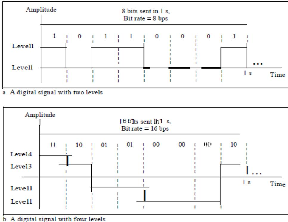
We send 1 bit per level in part a of the figure and 2 bits per level in part b of the figure. In general, if a signal has  $L$  levels, each level needs  $\log_2 L$  bits.
