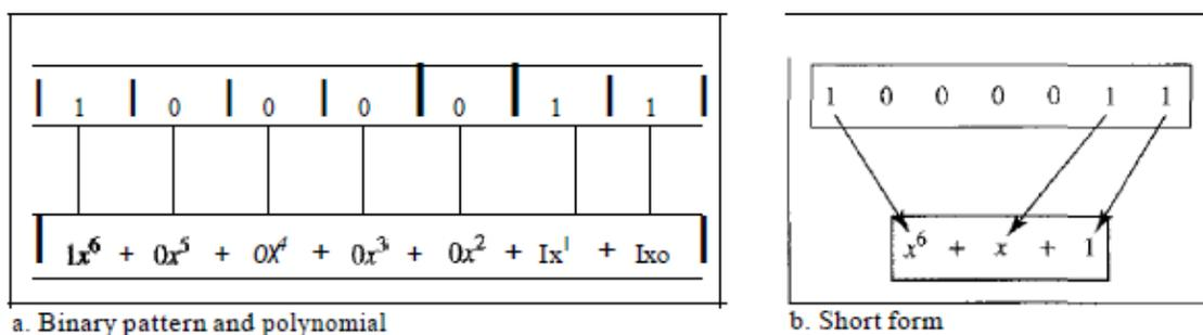
Figure 10.21 shows one immediate benefit; a 7-bit pattern can be replaced by three terms. The benefit is even more conspicuous when we have a polynomial such as  $x^{23} + x^3 + 1$ . Here the bit pattern is 24 bits in length (three 1s and twenty-one 0s) while the polynomial is just three terms.
