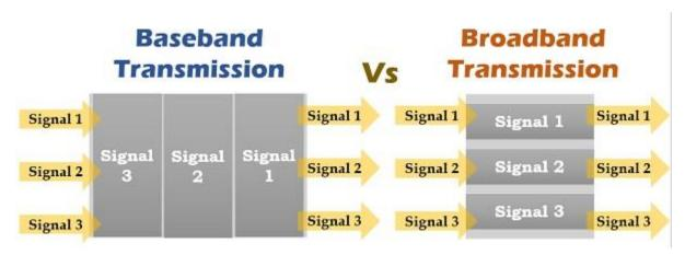
The baseband and broadband are the types of signaling techniques. These terminologies were developed to categories different types of signals depending on particular kind of signal formats or modulation technique.
