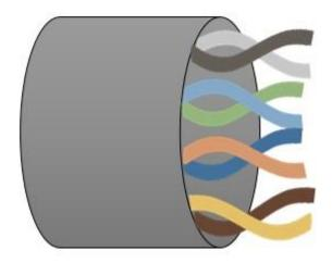
The two wires are twisted in the twisted pair cable which significantly reduces the noise generated by the external source. The **NOISE** here we are talking about is generated when two wires are parallel which causes an increase in
