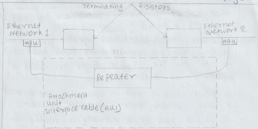
MAU (medium Attachment unit) and AUI can be optionally combined in a single unit with the Repeater.
