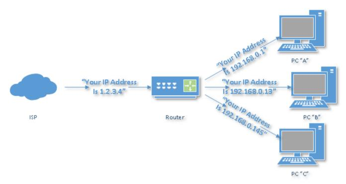
IP address assignments to and through a router.
