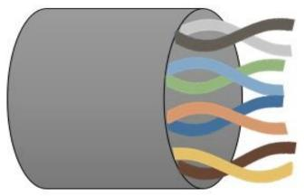
**Shielded twisted-pair (STP) cable** has an additional braided mesh coating or metal foil that wraps each set of insulated conductors. The metal casing intercepts the penetration of **electromagnetic noise**. It also can eradicate a phenomenon called crosstalk, which is the unwanted effect of one circuit (or channel) on another circuit (or channel).
