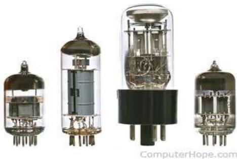
The first generation of computers used [vacuum tubes](#) as a major piece of technology. Vacuum tubes were widely used in computers from [1940](#) through [1956](#). Vacuum tubes were larger components and resulted in first-generation computers being quite large in size, taking up a lot of space in a room. Some of the first-generation computers took up an entire room.
