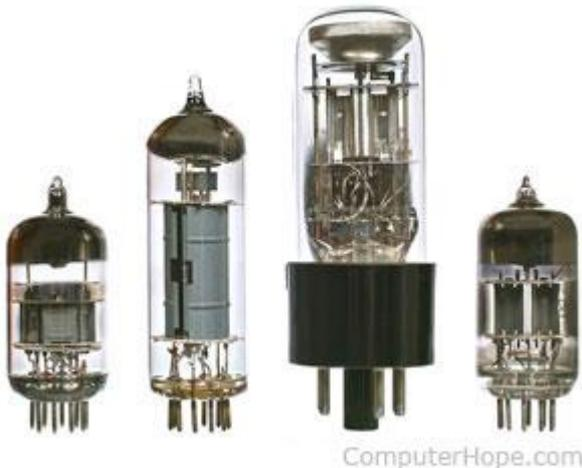
The first generation of computers used [vacuum tubes](#) as a major piece of technology. Vacuum tubes were widely used in computers from [1940](#) through [1956](#). Vacuum tubes were larger components and resulted in first generation computers being quite large in size, taking up a lot of space in a room. Some of the first generation computers took up an entire room.
