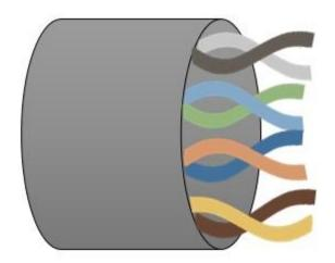
The two wires are twisted in the twisted pair cable which significantly reduces the noise generated by the external source.
