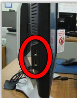
4. **Fit** the connector into the port and **push** it in gently.
