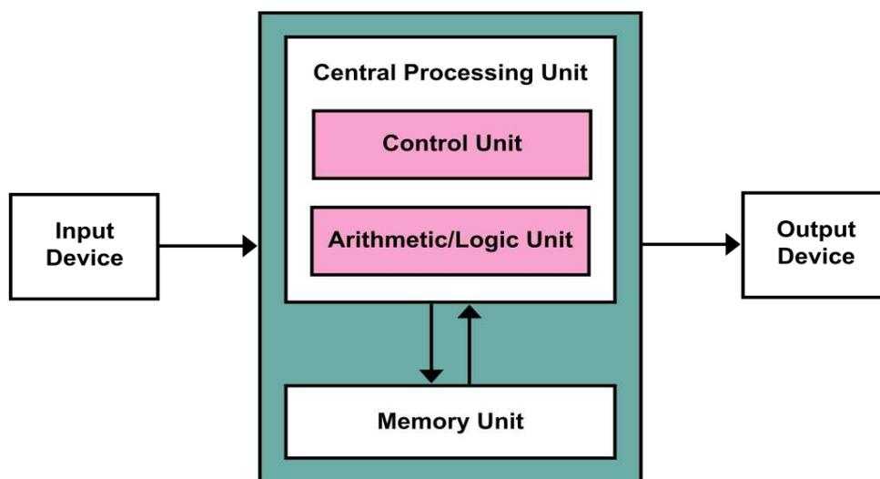
**Input Devices:** Computer systems use many devices for input purpose. Input devices include the mouse, input pen, touch screen, and microphone. Regardless of the type of device used, all are components for interpretation and communication between people and computer systems.
