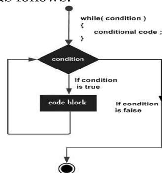
The above code can be represented in the form of a flow diagram as shown above
