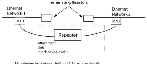
MAU (Medum Attachment Unit) and AUI can be optionally combined in a single unit with the Repeater
